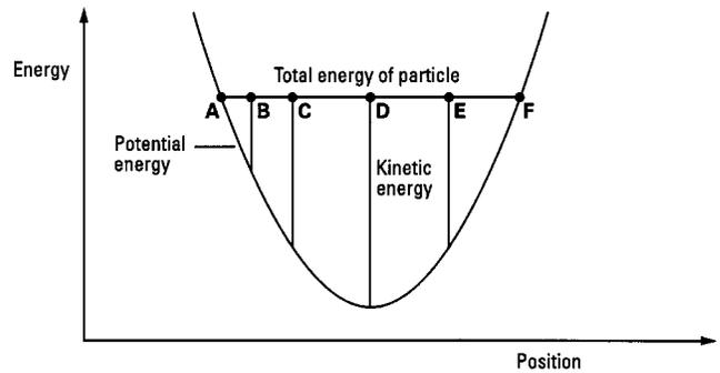
Fig. 1. The potential energy diagram is central to our treatment and requires a difficult conceptual progression from a ball rolling down a hill pictured in an  $x$ - $y$  diagram to a graphical point moving along a horizontal line of constant energy in an energy-position diagram. Making this progression allows the student to describe qualitatively, but in detail, the motion of a particle in a one-dimensional potential at arbitrary positions such as A through F.
