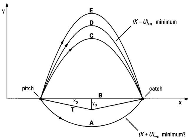
Fig. 6. Alternative trial trajectories of a pitched ball. For path D the average of the difference  $K - U$  is a minimum.
