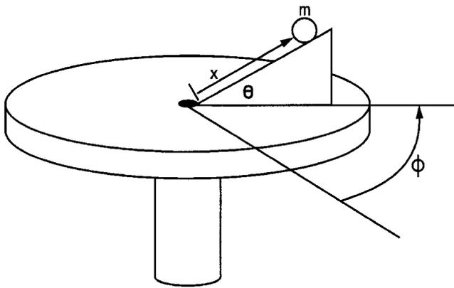
Fig. 3. System of marble, ramp, and turntable.
