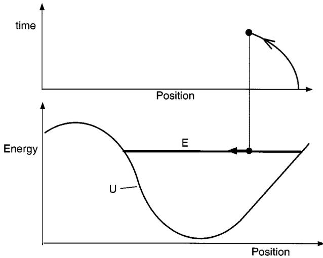
Fig. 2. Mockup of an interactive computer display of the worldline derived numerically from the energy and the potential energy function.
