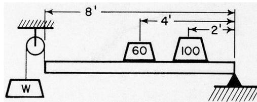
Fig. 4. Feynman's example of the principle of virtual work.
