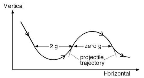
FIGURE 2 Trajectory followed by the Vomit Comet airplane above Earth's surface. Portions of the trajectory marked "2 q" and "zero q" are parabolas. During the zero-g segment, which lasts up to 30 seconds, the plane is guided to follow the trajectory of a free projectile in the absence of air resistance. By guiding the plane through different parabolic trajectories, the pilot can (temporarily!) duplicate the gravity on Mars (one-third of g on Earth) or the Moon (one-sixth of g on Earth).
