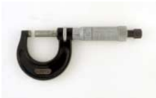
Figure 8 A micrometer caliper, used to measure small distances, such as the thickness of metal sheet. A calibrated screw on the right meters the gap between cylinders at the left.
